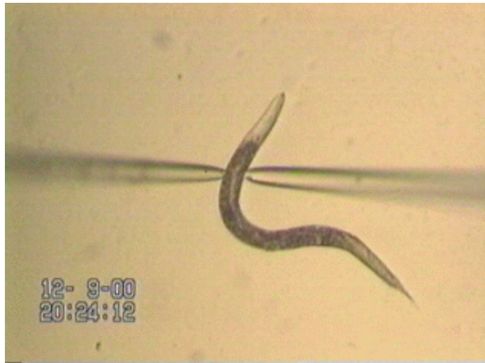
Figure 2.7: The video freeze image shows the procedure how to capture a living worm between two electrodes on the bottom of the petri dish for further treatment.
